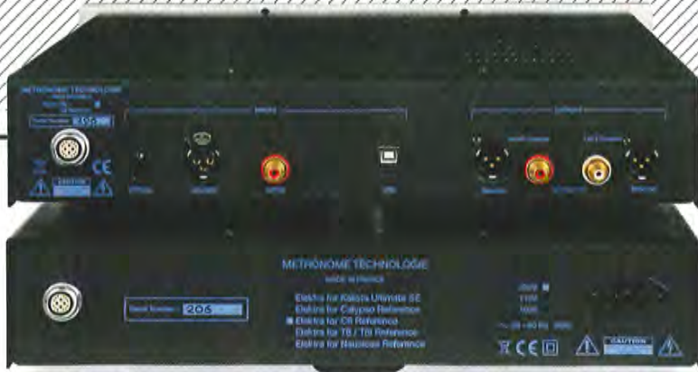
ABOVE: USB plus optical and coaxial S/PDIF and AES/EBU digital inputs with balanced (XLR) and single-ended (RCA) analogue outs. PSU connects via umbilical
